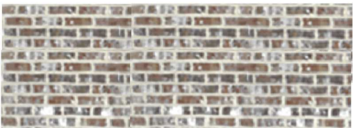
① Grey red washed brick with grey grout Provide sample to match
